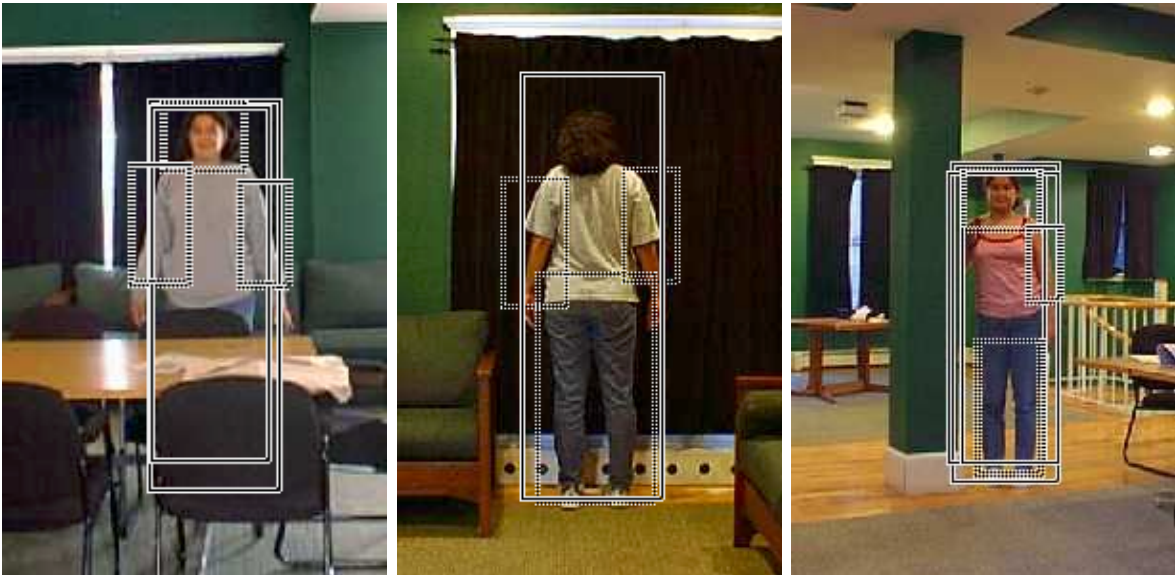
Figure 9: Results of the system's application to images of partially occluded people and people whose body parts have little contrast with the background. In the first image, the person's legs are not visible; in the second image, her hair blends in with the curtain in the background; and in the last image, her right arm is hidden behind the column.
