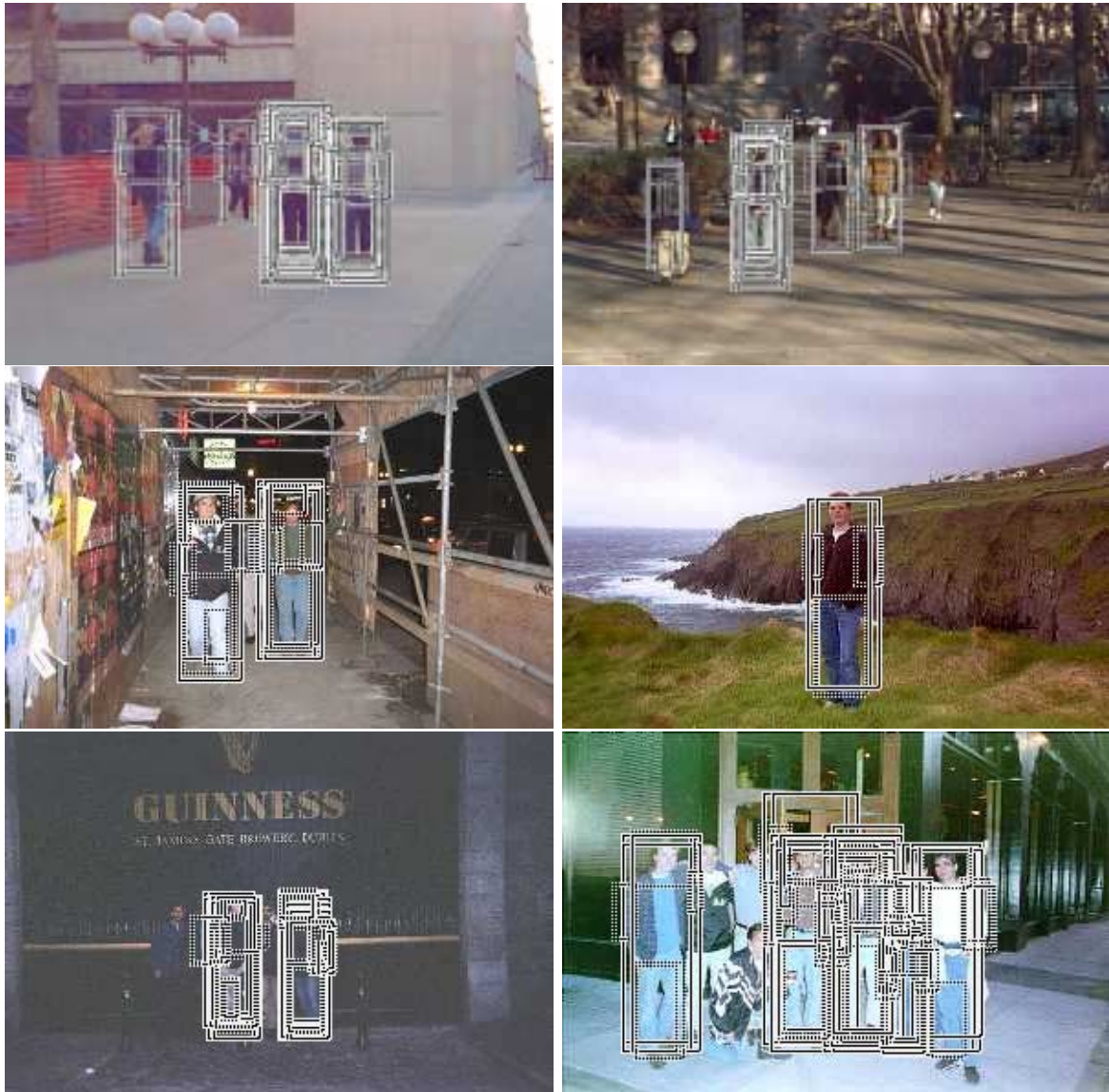
Figure 10: Results from the component based person detection system. The solid boxes outline the complete person and the dashed rectangles identify the individual components. People may be missed by the system because they are either too large or too small to be processed by the system (top right - person on the right); because several parts of their body may have very little contrast with the background (bottom left - person on the left) or because several parts of their body may be occluded (bottom right - person second from the left).
