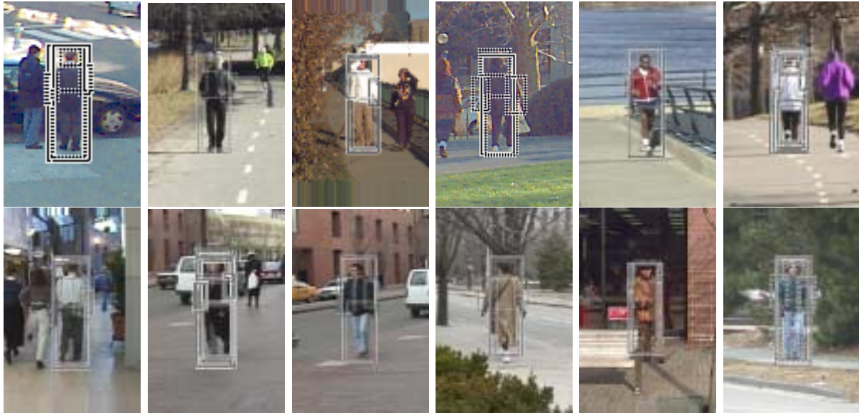
Figure 8: Samples from the test image database. These images demonstrate the capability of the system. It can detect running people, people who are slightly rotated, people whose body parts blend into the background (bottom row, second from right - the person is detected even though the legs are not), and people under varying lighting conditions (top row, second from left - one side of the face is light and the other dark).
