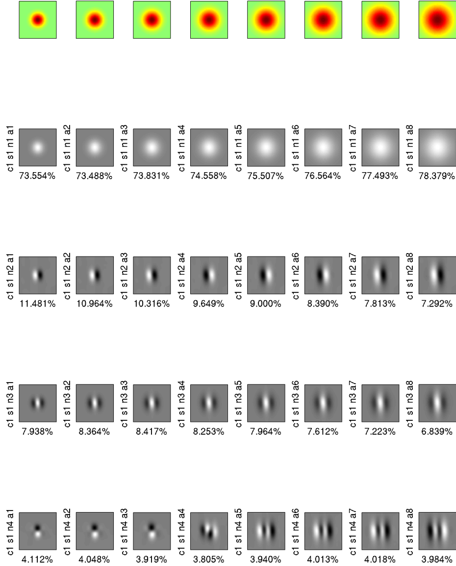
Figure 23: Principal components of the template book. These are obtained using the pipeline described in Figure 19. The pipeline consists of a Gaussian blur, a DoG filter, a spatial low-pass filter 1/\sqrt{\omega_x^2 + \omega_y^2} and an imperfect temporal derivative. The principal components are sorted by eigenvalue (row), different columns refer to different apertures of the receptive field.
