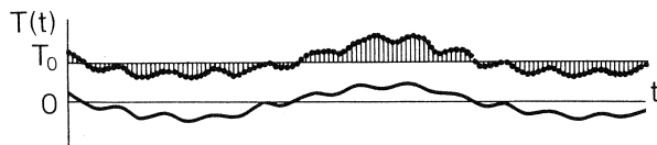
Fig. 3. The input x(t) consists of two sinusoidal waves with amplitude A_1 = 0.6 , A_2 = 0.3 and frequencies \omega_1 = 0.6 , \omega_2 = 5 . All other parameters are as in Figure 2. The maximum modulation amounts to 60%
