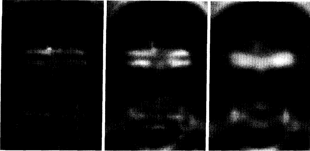
Fig. 6. The output of the correlation with an SDF computed using the spectral envelope of 10 training images and different amounts of white noise (left: \alpha=1 , middle \alpha=5 ) compared to the output of normalized cross-correlation using one of the images used to build the SDF but without any spectral enhancement. The darker the image the higher the corresponding value.
